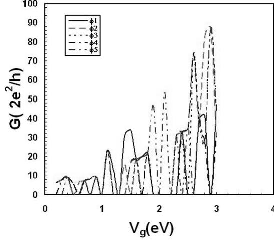
Fig. 3. The conductance-gate voltage dependence for different values of phase angle  $\phi$ .
