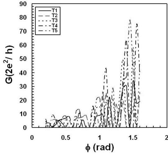
Fig. 4. The conductance-phase angle dependence for different values of temperature  $T$ .
