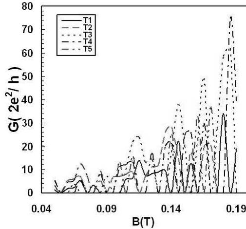
Fig. 2. The conductance-magnetic field dependence for different values of temperature  $T$ .
